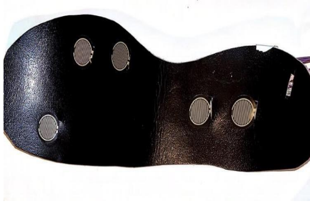
Figure 1b. Placement of FSR
