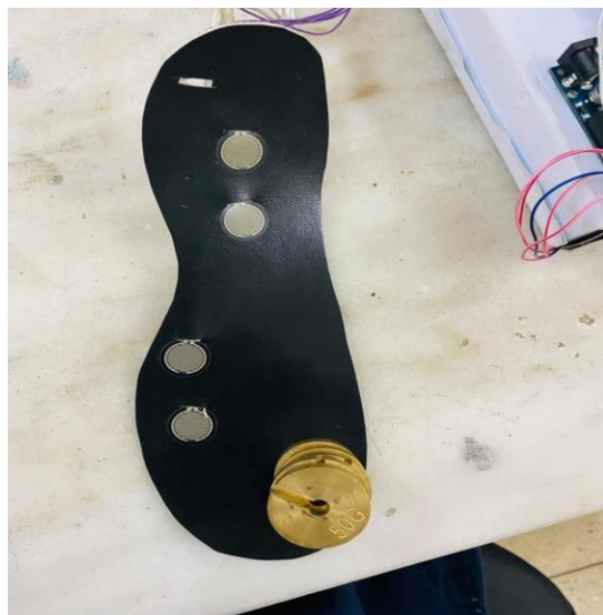
Figure 6. Calibration using known weights
